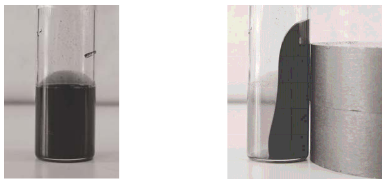
Figure 1. Example of an iron oxide dispersion in zero-field (left) and exhibiting the equilibrium shape in a field gradient typical for ferrofluids (right).
